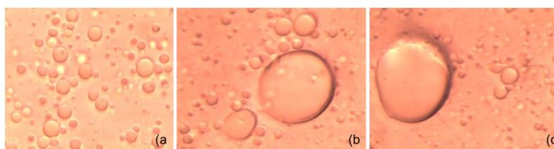
**Fig. 5** Optical microscope images of o/w GAPs emulsion; (a) without thermolysin, (b,c) after adding 1.5 mg/mL thermolysin.
